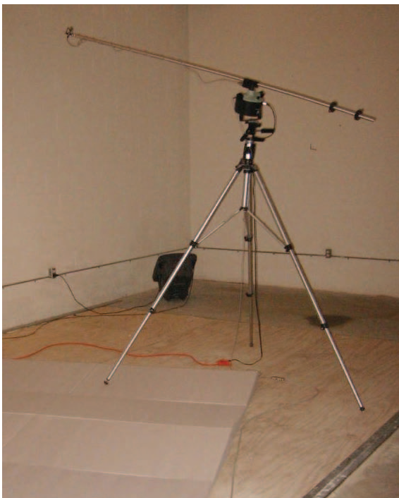
Figure 17 – Noise Reduction Coefficient (NRC) testing of acoustical wall panel
